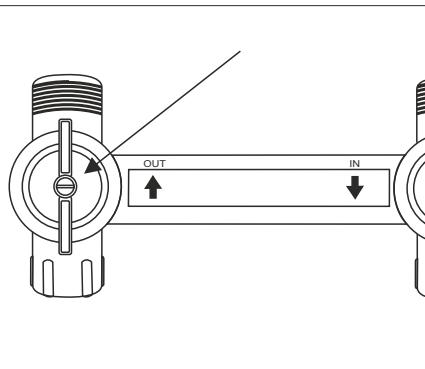
STEP 1. Adjust the residual hardness of the water that leaves the appliance, by means of the adjusting screw, incorporated in the 'outlet' valve of the factory bypass:
