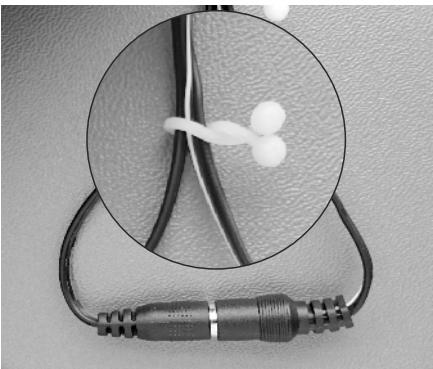
STEP 1. Plug the transformers output lead into the socket on the appliances power cord; secure it by means of the TwistLock clamp.
