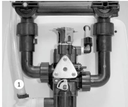
STEP 1. Connect a 13 mm hose to the drain solenoid of the control valve (1); secure it by means of a clamp.
